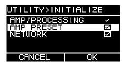
3. Turn the main knob to choose the type of settings that will be initialized (multiple selections are possible), and press the main knob to confirm.
