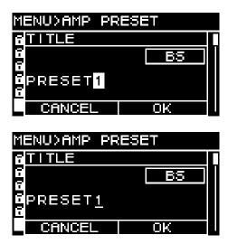
Turn the main knob to select the position at which to edit a character, and then press the main knob to enter character input mode. In character input mode, turn the main knob to select the character that you want to input, and then press the main knob to confirm the character.
