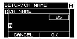
In character input mode, turn the main knob to select the location at which you want to input a character, and then press the main knob to confirm. Turn the main knob to select the character that you want to input, and then press the main knob to confirm the character.
