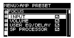
You can select multiple parameters as the object of focus. You can't modify an amp preset that is protected.
