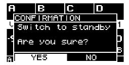
2. Turn the main knob to select "YES," and then press the main knob to confirm; the power switches to standby mode.
