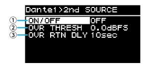
The backup circuit can be specified in two levels. The channel combinations are fixed.
