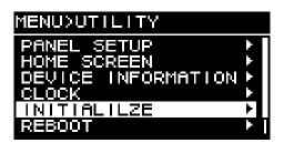
2. In the UTILITY screen, turn the main knob to select "INITIALIZE," and press the main knob to confirm. The INITIALIZE screen appears.
