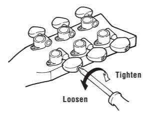
The tuning machines have spring-loaded mechanisms which automatically take up wear, preventing backlash. However, it is possible to adjust the amount of pressure required to turn the machines. Each machine has a tension adjustment screw, as illustrated.
