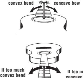
The curvature of the neck should be slightly concave. Clockwise rotation of the nut tightens the rod and corrects for too much concave bow. Counterclockwise rotation of the nut loosens the rod and corrects for too much convex bow. Make any adjustments gradually. Allow five to ten minutes for setting, and check the curvature after each 1/2 turn of the truss rod nut.
