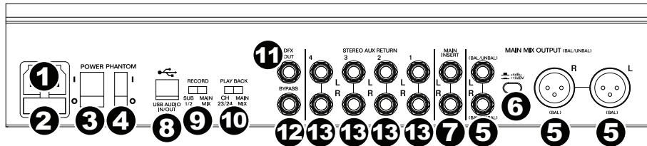
1. **Power In:** Use the included power cable to connect the mixer to a power outlet. While the power is switched off, connect the power cable into the mixer first, then connect the power cable to a power outlet.
