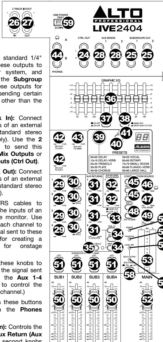
33. **Aux Return 3 Routing:** When this button is depressed, the signal sent into Aux Return 3 will be routed to the Control Room Mix. When this button is raised, the signal is sent to the Main Mix.
