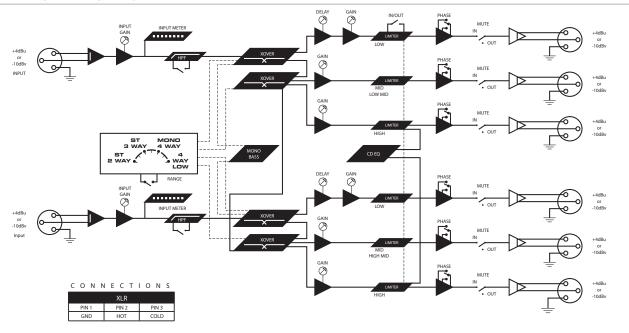
Modes Stereo 2 Way Stereo 3 Way Mono 4 Way Mono 4 Way Low Operating Frequencies Ch 1 A 35Hz to 800Hz X1 or 350Hz to 8KHz 35Hz to 800Hz X1 or 350Hz to 8KHz 35Hz to 800Hz 18Hz to 400Hz Operating Frequencies Ch 1B 350Hz to 8KHz 350Hz to 8KHz 350Hz to 8KHz 175Hz to 4KHz Operating Frequencies Ch 2 A 35Hz to 800Hz X1 or 350Hz to 8KHz 35Hz to 800Hz X1 or 350Hz to 8KHz Operating Frequencies Ch 2B 350Hz to 8KHz 350Hz to 8KHz 350Hz to 8KHz 700Hz to 8KHz
